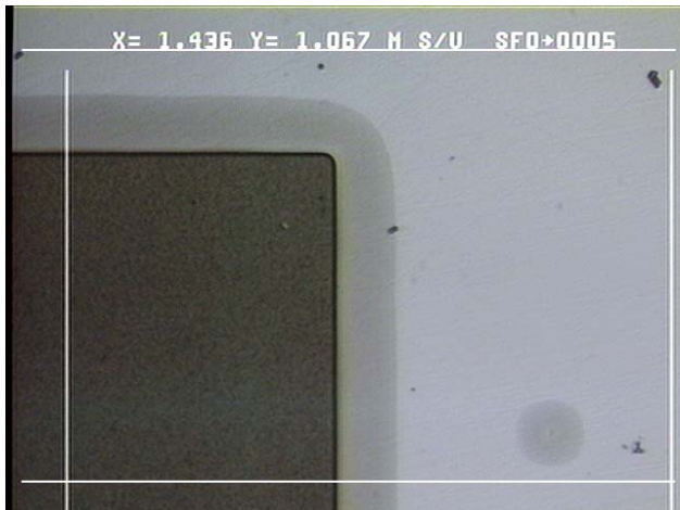
Coupling grating, spacing = 16\ \mu\text{m} , depth = 1.6\ \mu\text{m}
