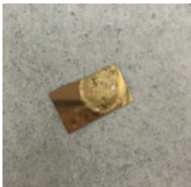
Figure 4. UiO-66 dropcast on Au coated Si wafer
