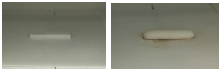
FIG. 3: A powder sample of \text{Li}_2\text{O} before sintering (left); the sample after sintering (right). The sample has expanded and lost its geometric shape. Craters are now present on its surface, and stains on the plate below indicate some amount of melting.
