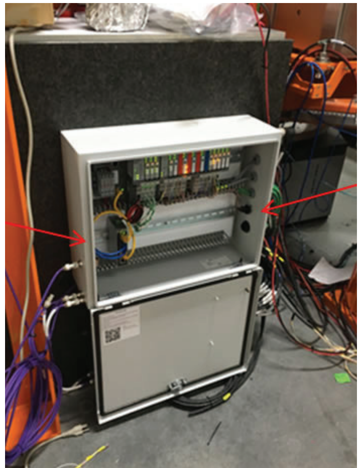
Image 2: The EPS box should have better ventilation where the arrows are directed.
