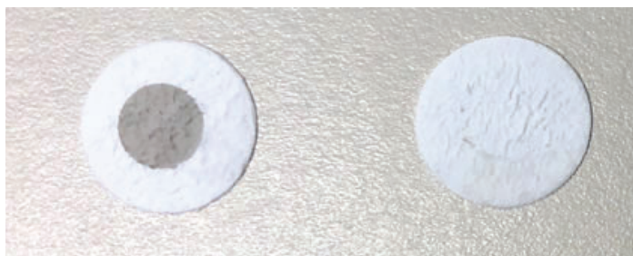
Figure 3. Example of a sample (left) and reference (right) PSAP filter.
