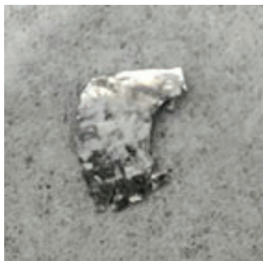
Figure 5. UiO-66 pressed into indium foil
