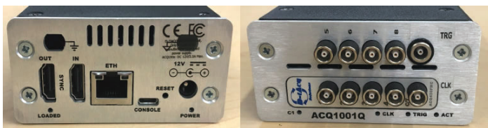
Figure 4- View of the front panel (left) and rear panel (right) of the ACQ1001-FMC digitizer
