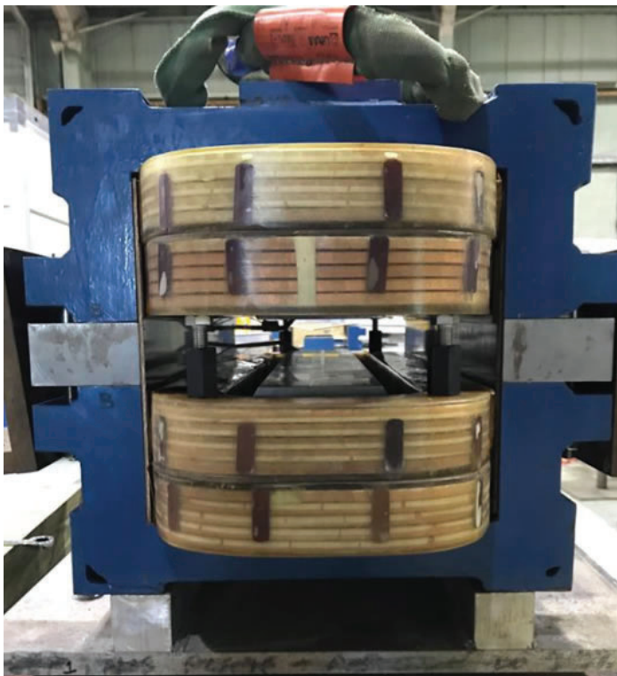
Figure 6: Photo of reconfigured dipole magnet showing gap and spacers
