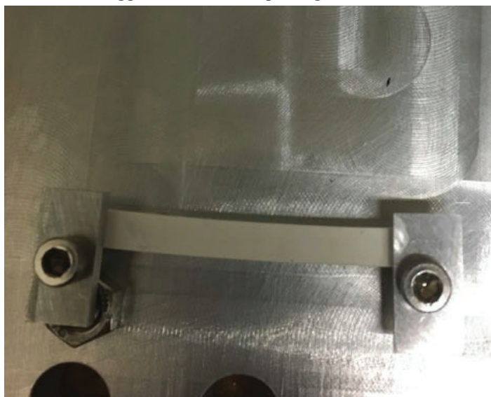
FIG. 4: Our first successfully baked \text{Li}_2\text{O} target pinned against a metal plate, as we prepare to install it into the laser chamber.
