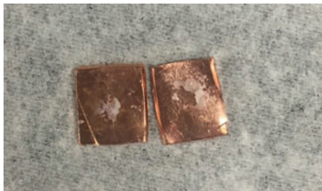
Figure 6. UiO-66 pressed between copper plates
