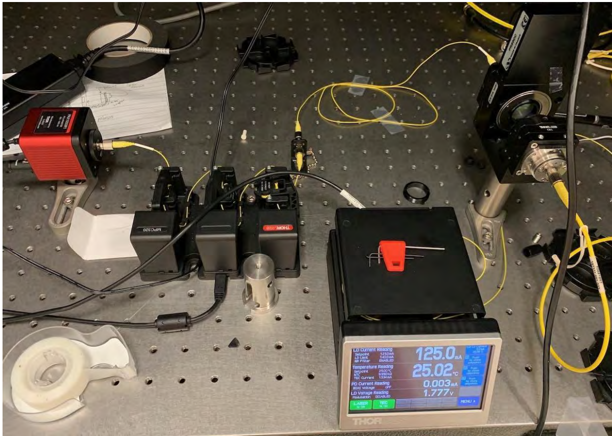
Image 2: The first test setup used to test the correction algorithm. The yellow fiber optic cable was twisted to change the effect of the channel on the incoming polarizations.
