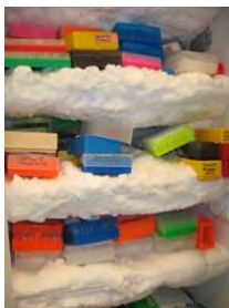
Figure 5: An example of a freezer with ice build up
