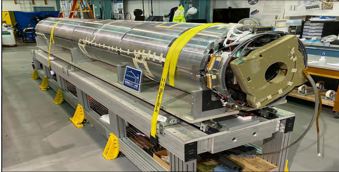
Figure 2: This shows a superconducting magnet used for the LHC upgrade.
