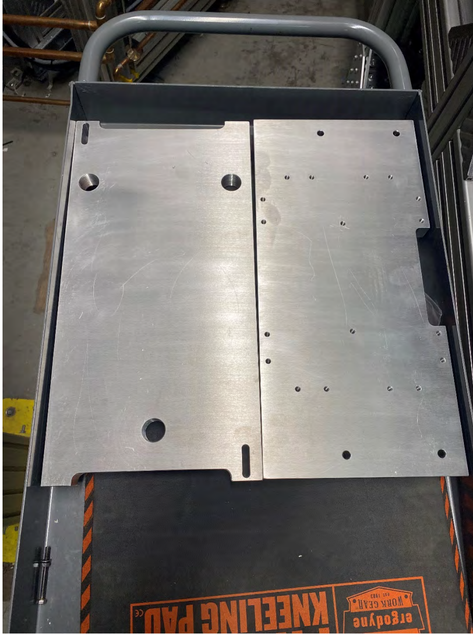
Figure 17: Manufactured Solenoid Plate (Left) and H/V Slit Plate (Right)
