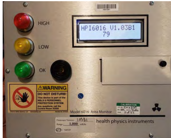
Figure 2 - HPI 6016 Area Radiation Monitor
