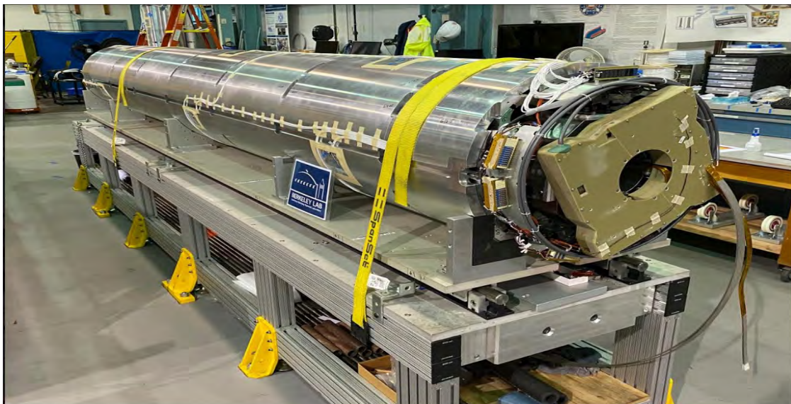
Figure 2: This shows a superconducting magnet used for the LHC upgrade.
