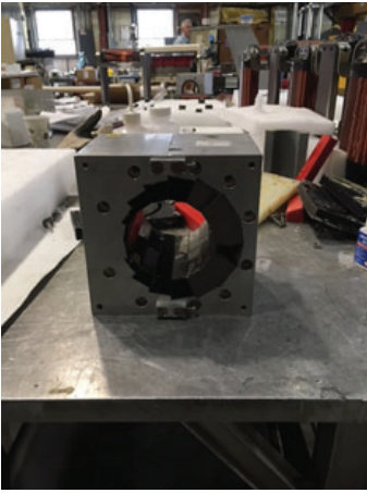
Figure 1. Completion of a working prototype of the Halbach dipole.
