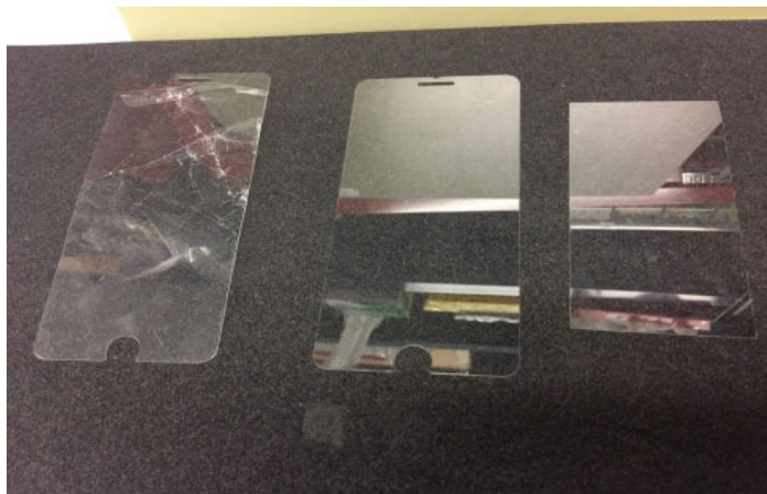
Figure 3: Glass Results (from left to right): 160 um glass after attempt at cutting, 160 um glass before, 200um glass after
