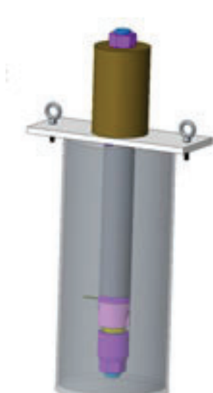
Figure 3- CAD model of compression fixture assembly
