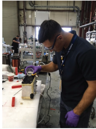
Figure 2. Epoxy is being poured into the vacuum fixture and being drawn
