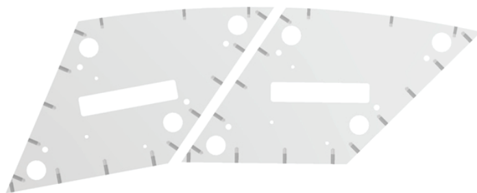
Figure 4: Splice plate hole spacing, the endplates of the two sectors and the placement of their holes and set screws.
