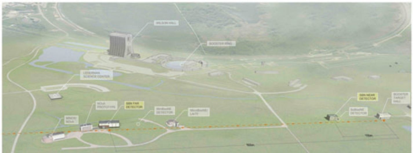
Figure 1: An aerial view of the MicroBooNE experiment. The beam travels from right to left along the dashed orange line. The MicroBooNE beam (BNB) is 470 m from the detector (LArTPC).
