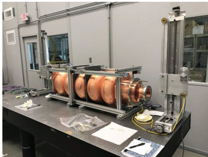
Figure 1: Current Bead-Pull Setup at BNL
