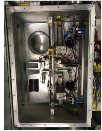
Figure 4. Diagnostic box with rails extended, note white and yellow 3D printed parts.
