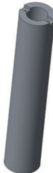
Figure 4- CAD model of thick walled compression tube
