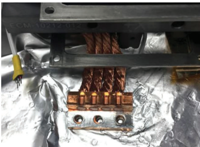
Figure 12: 0.01” indium foil cut and applied to thermal strap end
