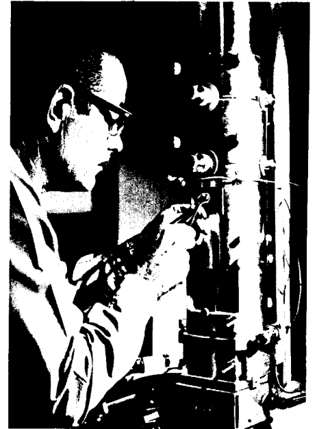
A metal sample is prepared for insertion into an electron microscope for metallographic examination in the Instrumentation and Health Physics Department. Besides the scanning machine, the Microscopy Laboratory has three transmission electron microscopes and several optical microscopes. The optical microscopes are used for preliminary examination of samples, and for precision mounting of specimens in the electron microscopes.
