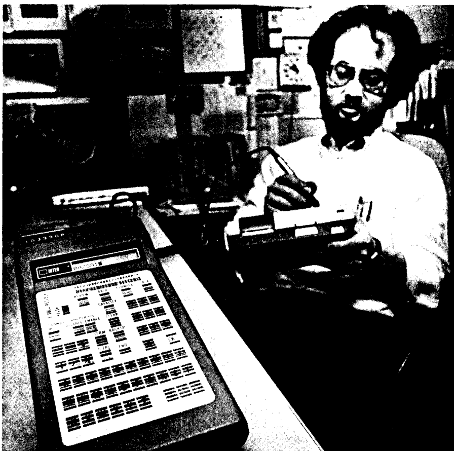
Alan Bieber demonstrates the use of a bar code reader to keep track of sensitive inventory.
