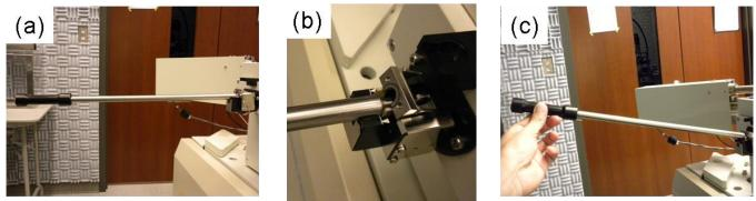
FIG. 8. Retracting exchange rod. (a) Fully retracted and resting on the plastic stopper. (b) Detail of rod resting on plastic stopper. C) Lifting of rod to its vertical position without using any force along rod's axis.
