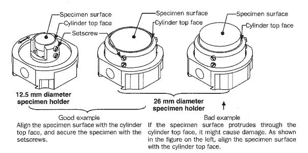
FIG. 1. Specimen positioning on 12.5 and 26 mm holders. (Diagram taken from JEOL's manual.)
