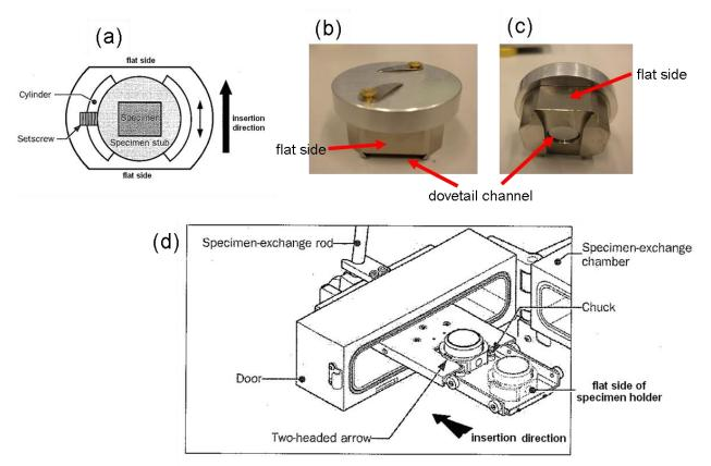
FIG. 4. Locking the sample holder in place in the airlock chamber. a) Top view of specimen holder. b) and c) Identification of "flat side" with respect to dovetail channel at the base of holder. The flat side is perpendicular to the length of the dovetail channel. d) Correct way of locking specimen holder with the holder's flat side perpendicular to the insertion direction. (Diagrams taken from JEOL's manual.)
