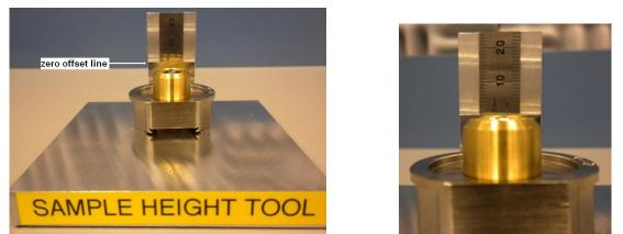
FIG. 2. Sample height tool. The right image shows a sample correctly flushed at the zero offset line.
