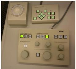
FIG. 11. Knobset panel, specimen stage control panel and trackball.
