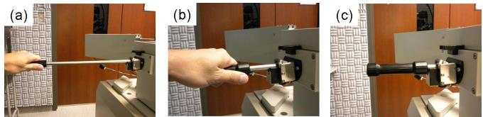
FIG. 7. Locking holder in SEM stage. (a) Insertion of rod by pushing horizontally along rod's axis. (b) Rod position when it first touches the SEM stage. (c) Rod position with holder locked in SEM stage.
