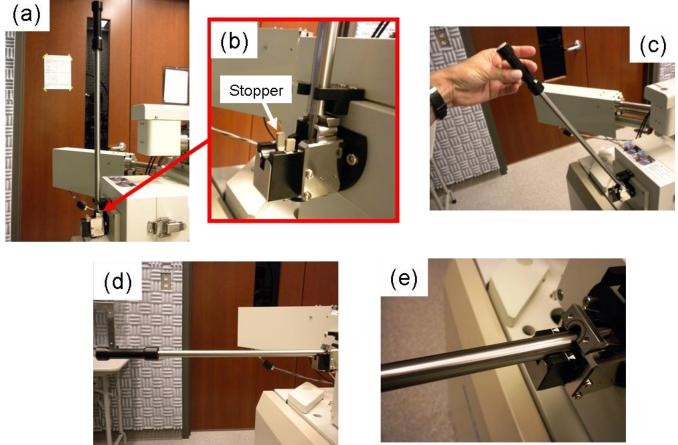
FIG. 6. Lowering of specimen-exchange rod. (a) Initial vertical position. (b) Detail of location of the plastic stopper. (c) Lowering of rod without pulling along its axis. (d) Fully horizontal position. Rod is held extended due to friction in sliding metal parts. Note that plastic stopper is pushed down when rod is horizontal as shown in (e).
