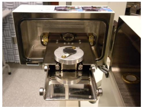
FIG. 5. Sample locked in place in the airlock chamber
