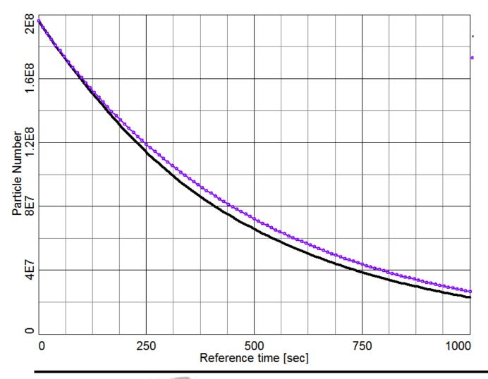
Results of optimization for June 2009 lattice and previous RF parameters (50kV).
