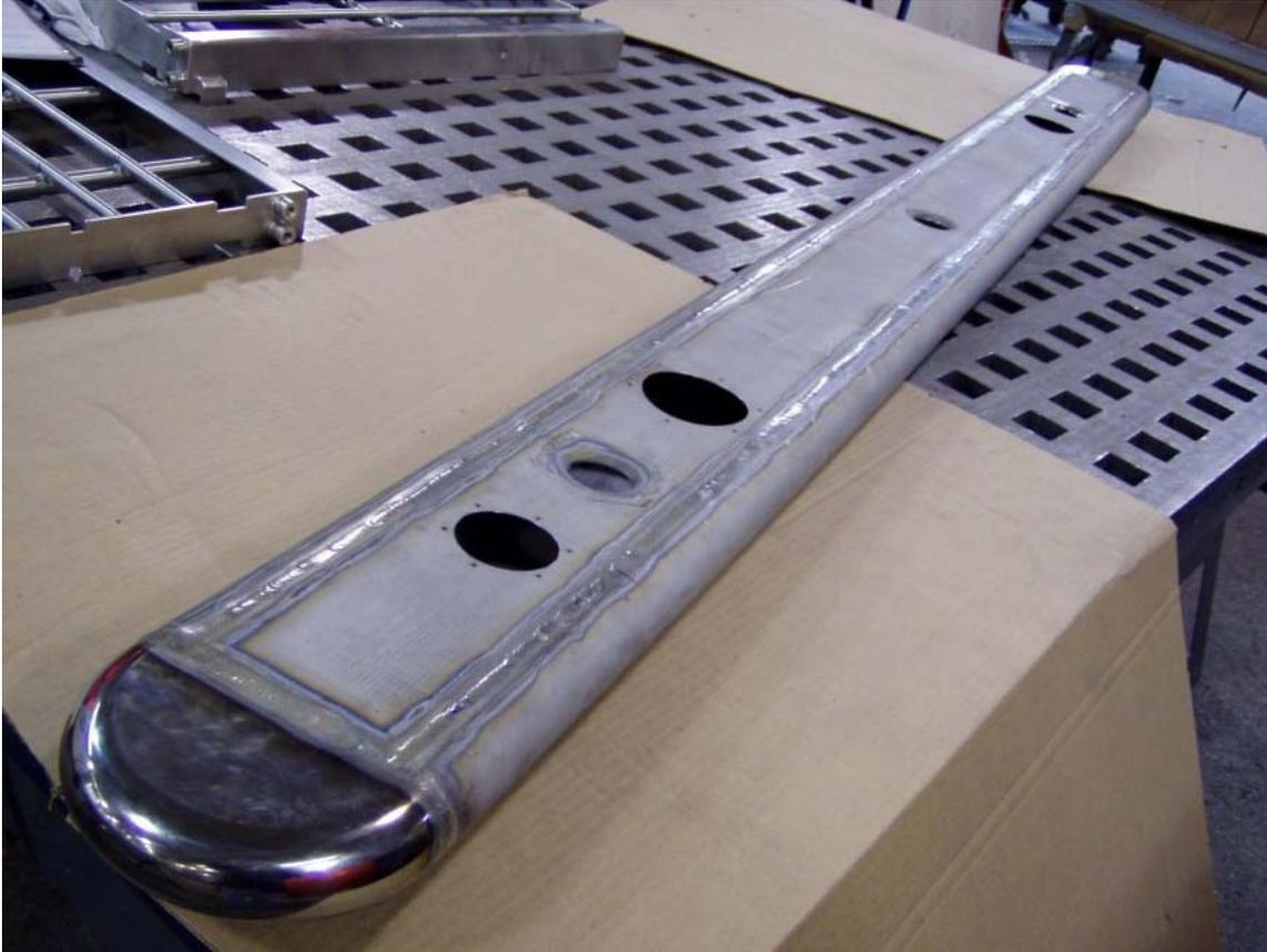
Fig. 4DS. Tevatron separator 101 inch long electrode during construction (back side).
