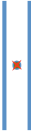
Figure 4. The vertical lines represent vertical electric field plates. The counter-rotating beams are indicated in the middle between the plates. Either electric or magnetic focusing systems are under consideration.
