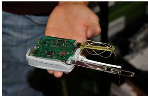
Radiosonde (sensor attached to a weather balloon that makes measurements and relays information). They don't work as well after hitting containers.
