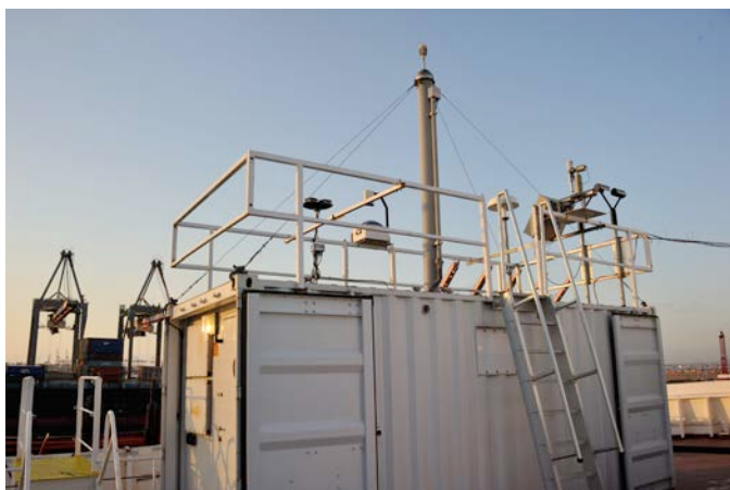
AOS with stack; other instruments are mounted on the roof railings
