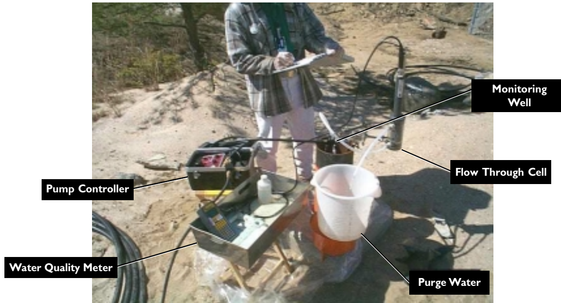
Figure 7-3. Sampling a Groundwater Monitoring Well.
