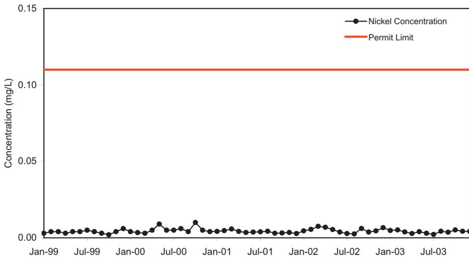
Figure 3-5. Maximum Concentration of Nickel Discharged from the BNL Sewage Treatment Plant, 1999–2003.
