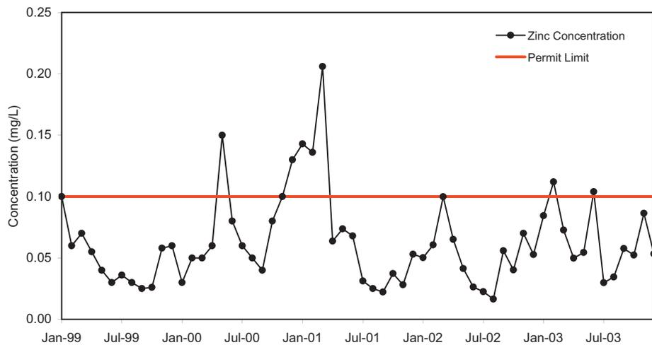
Figure 3-6. Maximum Concentration of Zinc Discharged from the BNL Sewage Treatment Plant, 1999–2003.
