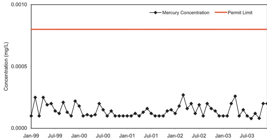
Figure 3-7. Maximum Concentration of Mercury Discharged from the BNL Sewage Treatment Plant, 1999–2003.
