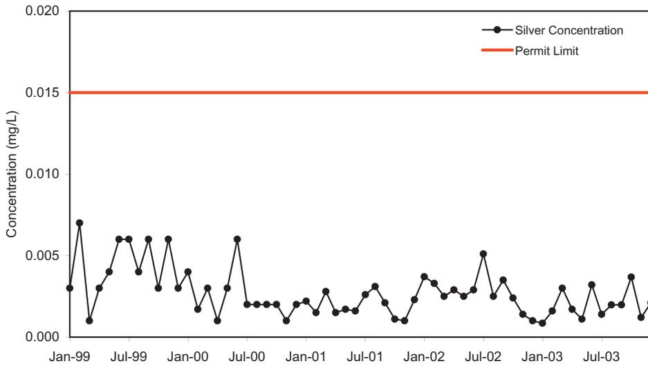
Figure 3-4. Maximum Concentration of Silver Discharged from the BNL Sewage Treatment Plant, 1999–2003.
