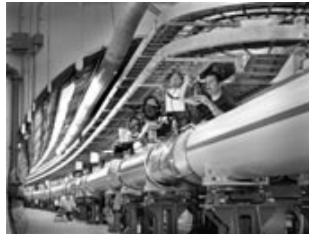
A view of the superconducting magnets at BNL's Relativistic Heavy Ion Collider. As gold particles zip along the collider's 2.4 mile long tunnel at nearly the speed of light, 1,740 of these magnets guide and focus the particle beams.
