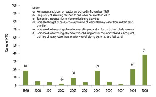
Figure 4-2. High Flux Beam Reactor Tritium Emissions, (1999–2009).
