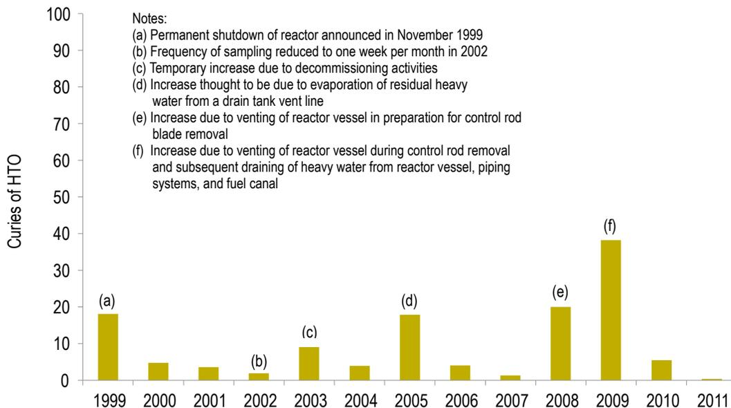
**Figure 4-2. High Flux Beam Reactor Tritium Emissions, Multi-Year Trend (1999–2011).**
