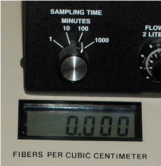
Readout after 100 minute sample event NOTE: decimal appears with three significant figures
