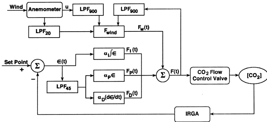
Fig. 3 FACE control algorithm schematic. Terms of the algorithm are in square boxes and are defined in the text. Round-edged boxes denote instruments receiving and/or sending signals to the control computer.
