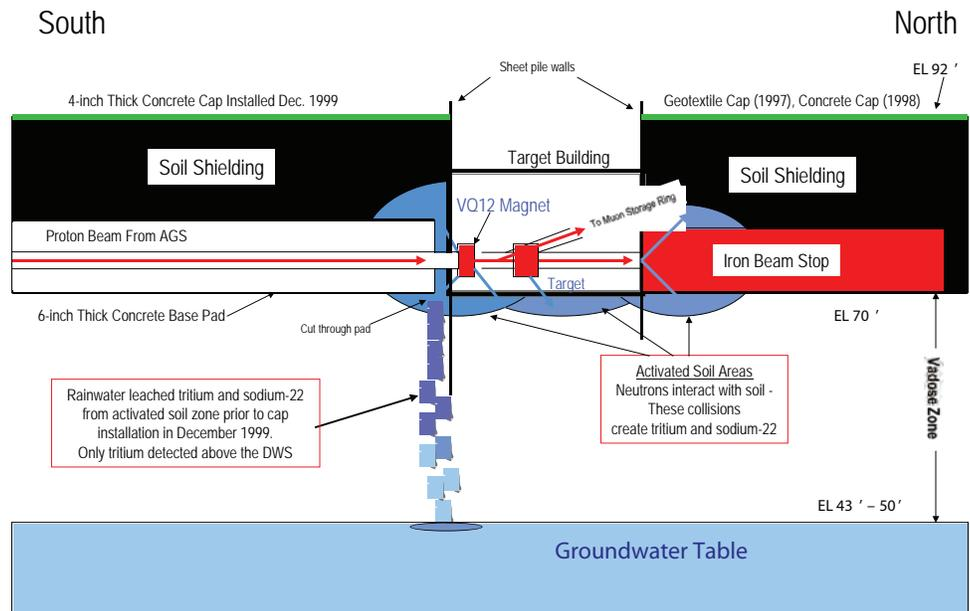
**FIGURE 2. Simplified cross section view of the soil activation area at the g-2 experiment.**
