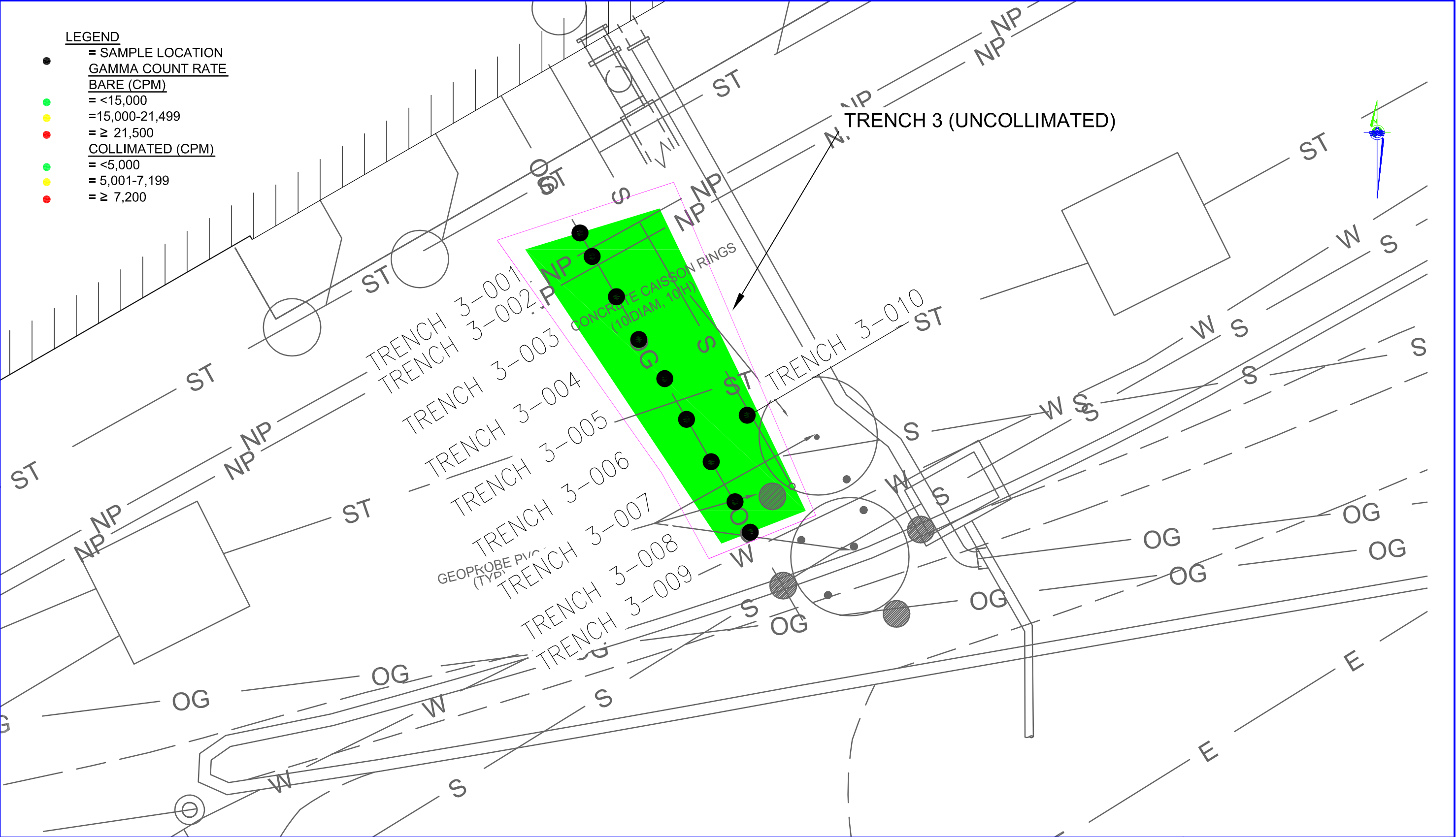
PHASE 3, TRENCH 3 FSS SAMPLE LOCATIONS AND RADIOLOGICAL WALKOVER SURVEY RESULTS
