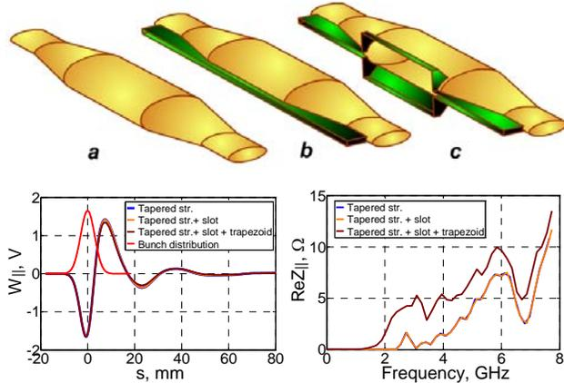
Figure 3: Simplified model of IR-extraction chamber. a) Tapered elliptic chamber. b) Tapered elliptic chamber with narrow slot. c) Tapered elliptic chamber with narrow slot and trapezoidal slot. **Left Bottom:** The longitudinal short-range wakepotential for a 3mm Gaussian bunch. **Right Bottom:** The real part of the longitudinal impedance.
