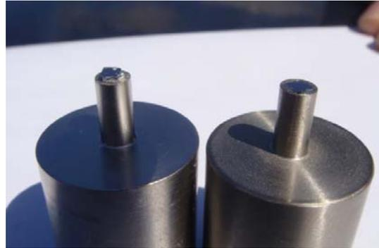
Figure 1: The cathode plug with original and recessed GaAs crystal.
