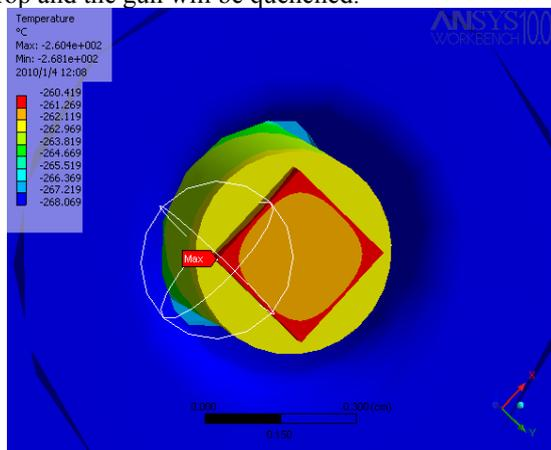
Figure 5: Temperature distribution at 5 MV/m, calculated with ANSYS. The picture shows the cavity walls (blue), the tip of the plug (yellow) and the GaAs crystal (orange/red).
