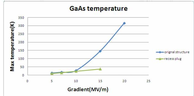
Figure 5: The GaAs crystal temperature simulation with two kind of plug designing.
