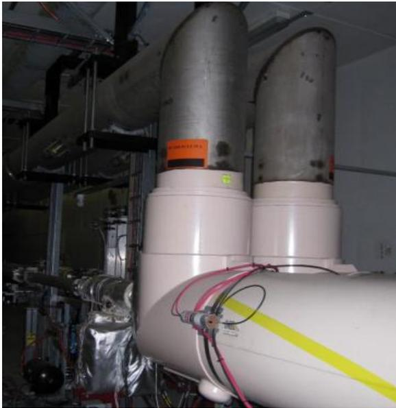
Fig. 2: A Typical Connection between Magnet Cryostat and Transfer Line VJP
