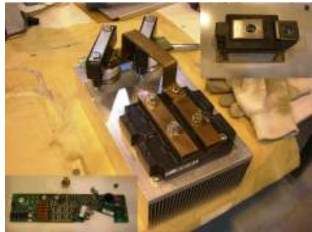
Figure 5: Power IGBT, SCR, Diodes and IGBT Driver
