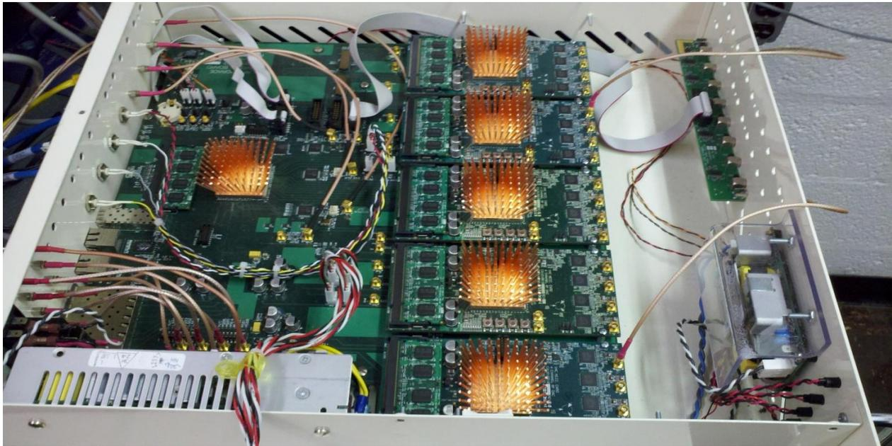
Figure 1: RF Controller Chassis populated with 5 XMC cards.
