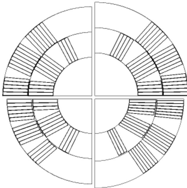
Cross-sections of coils with bore diameter of 40-50 mm
