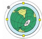
Several Nb<sub>3</sub>Sn short dipole models were fabricated and tested to demonstrate the possibility to reach the field >10 T at 4.3 K.
