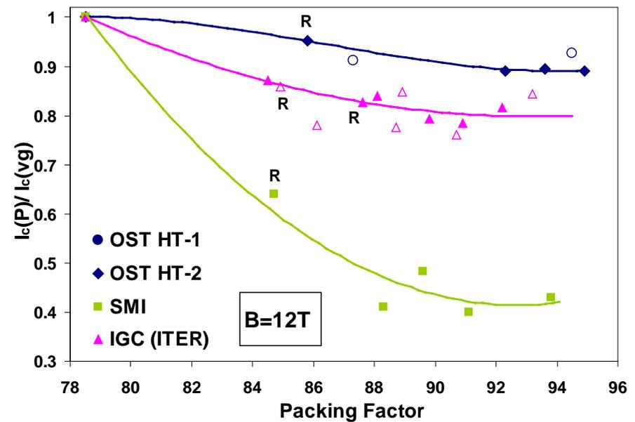
$I_c$  degradation vs. cable packing factor @ 12 T
