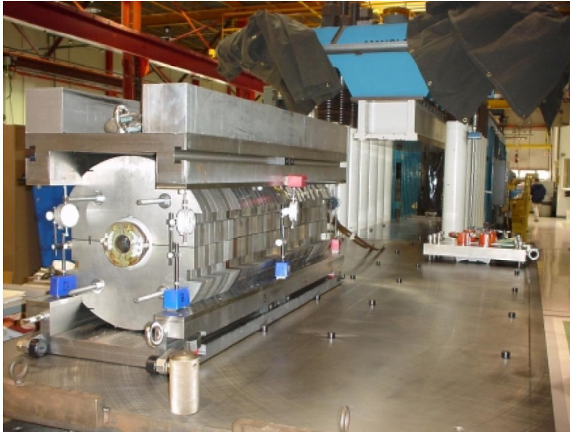
Short model assembled with iron yoke
