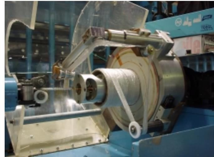
Cable insulation using the Insulation Wrapping Machine
