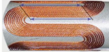
Figure 2. Serpentine style octupole coil pattern wound with five and a half turns per pole.
