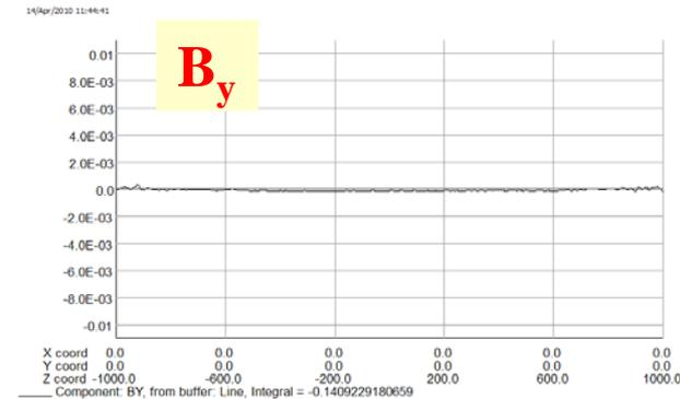
Works really well – even better than optimum integral design (field is very flat in this case).
