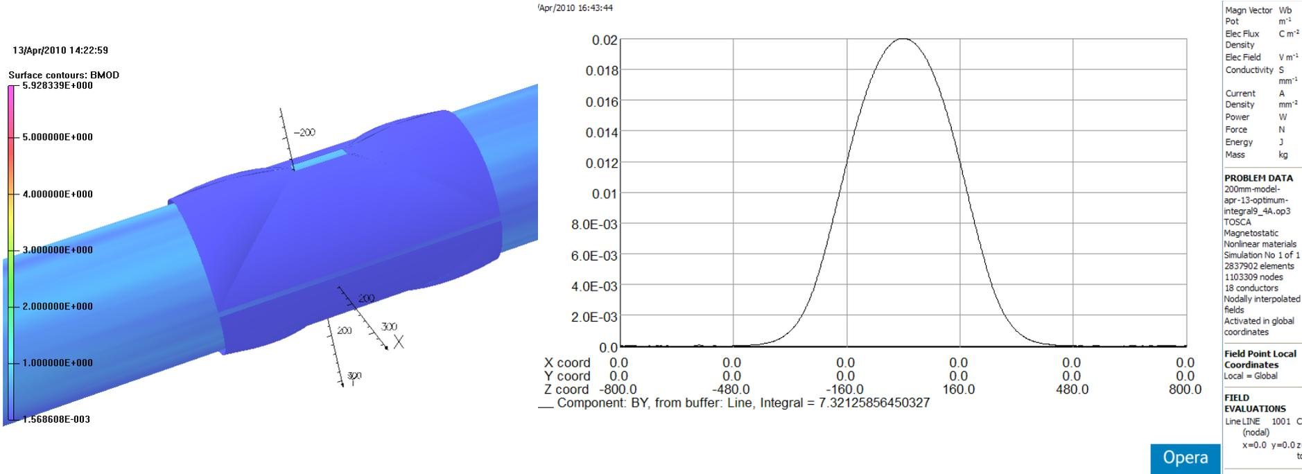
**Desired Field of 20 mT (0.02 T) is obtained at 9.4 A**
