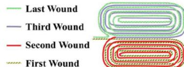
Figure 3. Pseudo-planar dual-layer winding pattern.
