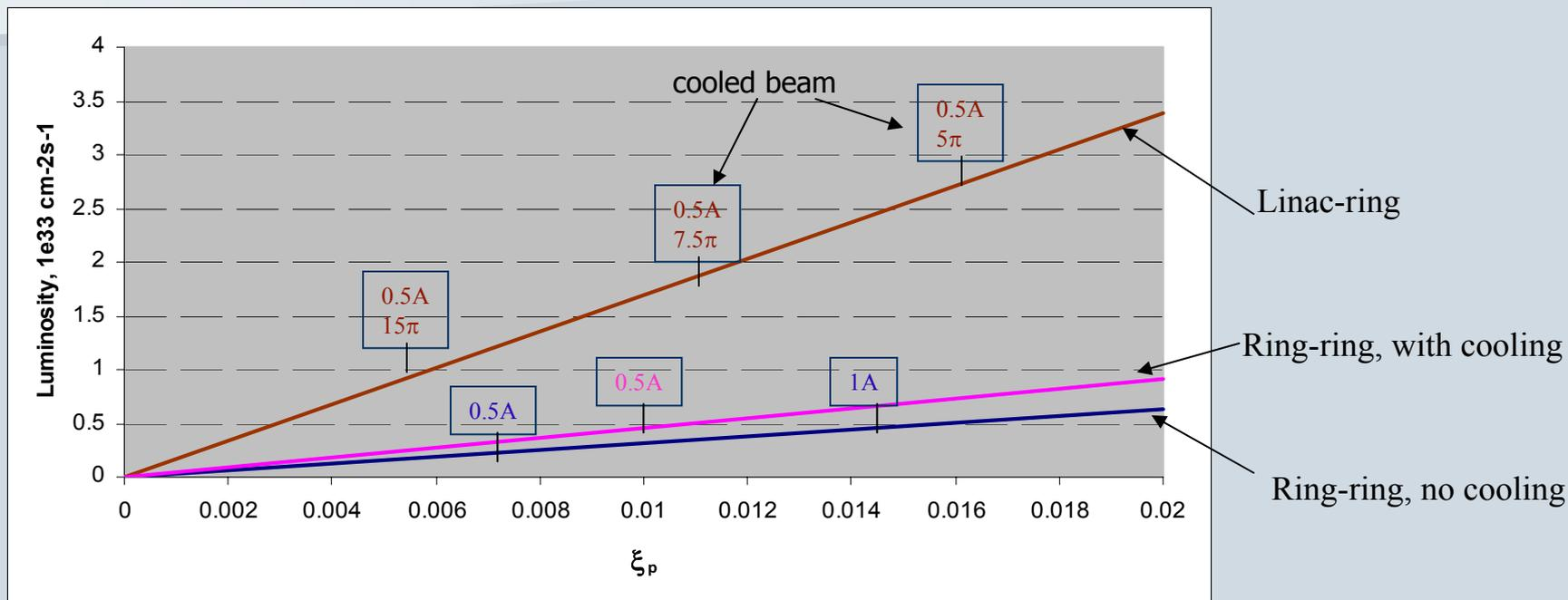
Markers show electron current and (for linac-ring) normalized proton emittance. In dedicated mode (only e-p collision): maximum  $\xi_p \sim 0.016-0.018$ ;
