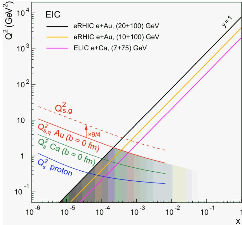
**Figure 12.** The quark saturation scales in gold and calcium at  $b=0$  and the median quark saturation scale in the proton are shown superposed on the kinematic EIC  $x$ - $Q^2$  acceptance. The gluon saturation scale is larger than the quark saturation scale by the color factor  $9/4$ .
