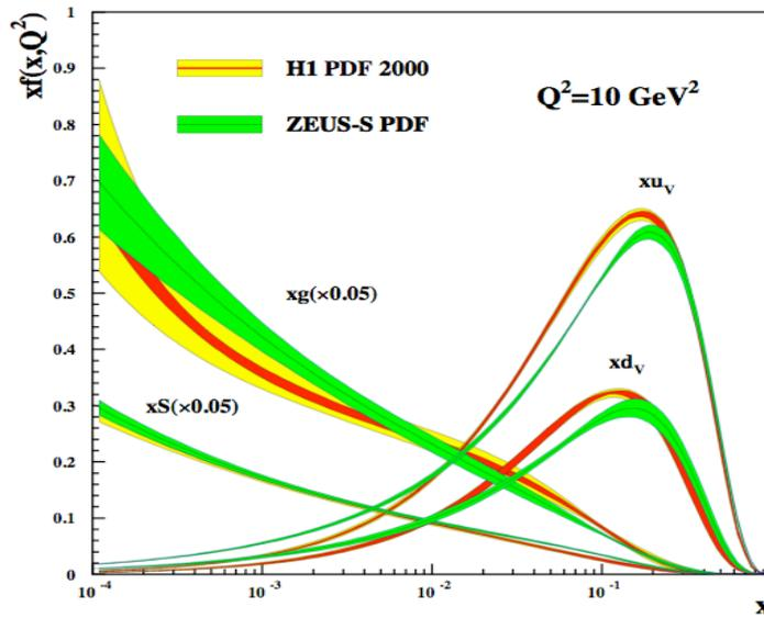
Figure 1. Quark and gluon distributions (valence quark  $u_V(x)$ ,  $d_V(x)$ ; sea quark  $S(x)$ ; gluon  $g(x)$ ) at  $Q^2 = 10 \text{ GeV}^2$  as determined at HERA by the H1 and ZEUS experiments [2]. Note the dominance of the gluon and sea quark distributions below  $x \sim 0.1$ .
