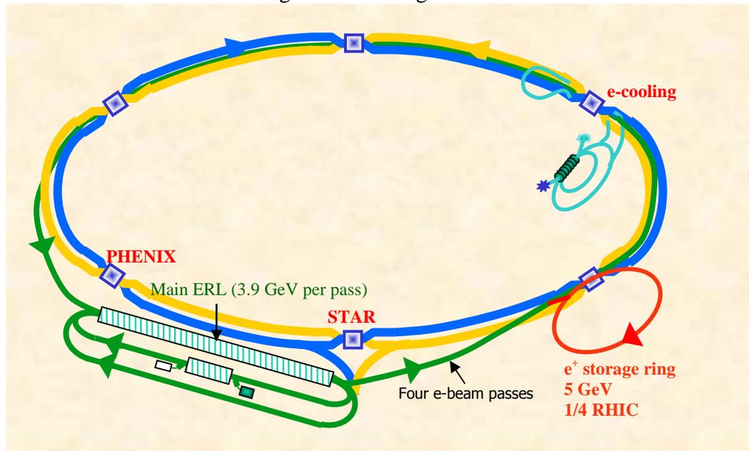
Figure 2.1: Design layout of the eRHIC collider based on the Energy Recovery Linac.
