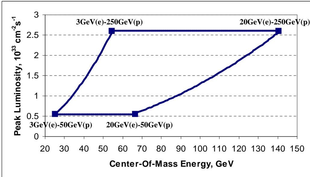
Figure 2.2. Luminosity scaling with the center-of-mass energy of eRHIC for e-p collisions.
