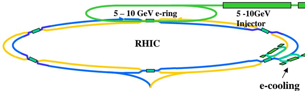
Figure 3.1: Design layout of the eRHIC ring-ring collider.
