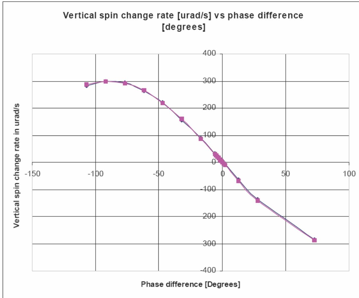
Figure 1. The vertical spin precession rate in  $\mu\text{rad/s}$  versus the phase difference ( $\phi$ ) between the synchrotron oscillations and the g-2 precession in degrees (modulo  $180^\circ$ ) for an RF-cavity offset of  $10\mu\text{m}$  is shown. An overlay of the function  $300 \mu\text{rad/s} * \sin(\phi)$  is also shown.
