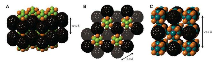
Space-filling structure of solidstate compound 1•2C60, showing the crystal packing looking along (A) the ab plane and (B) down the c axis. (C) Space-filling structure of 3•C60. Carbon, black; nickel, red; cobalt, blue; phosphorus, orange; tellurium, teal; selenium, green. The ethyl groups on the phosphines were removed to clarify the view.
