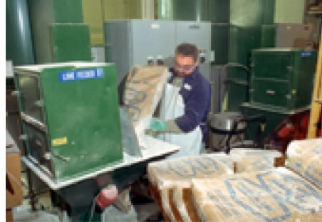
4. LIME is added after aeration (no. 3) and before retention (no. 6) to raise the pH and soften the water. Feeding lime into the hopper is Steve Barcelo.
