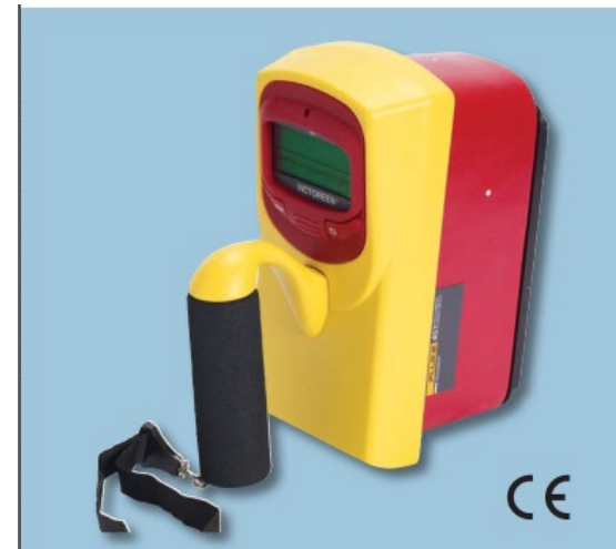
Ambient dose ion chamber for active dose measurements
