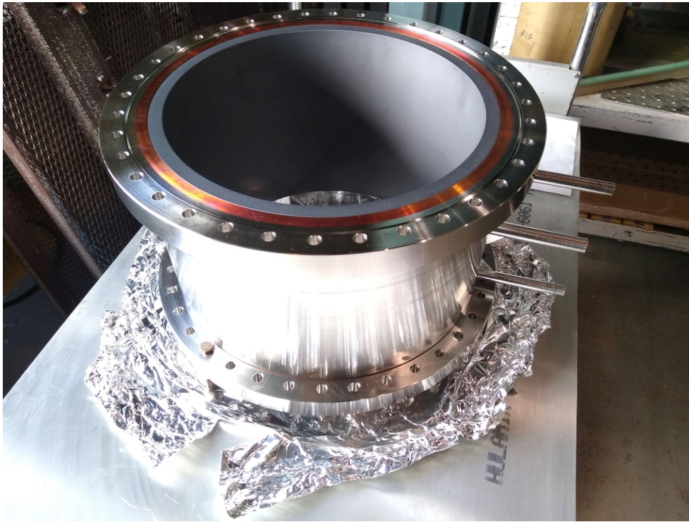
Figure 6.156: Fully assembled prototype SiC Beamline HOM Absorber (BLA).
