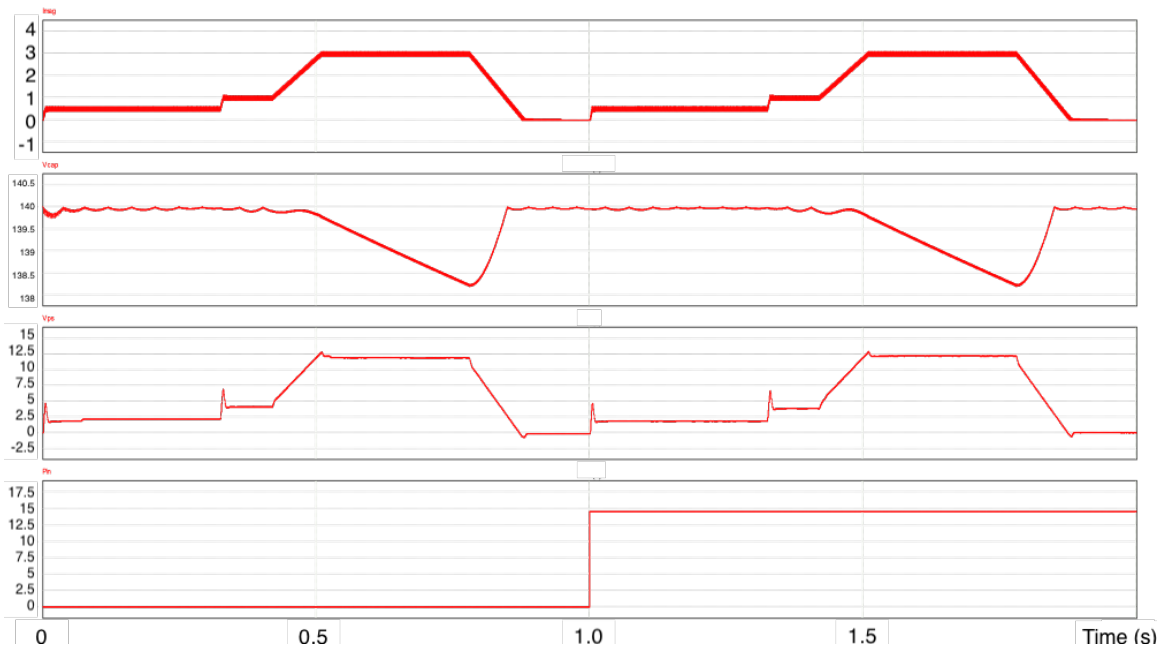
Figure 6.121: 5 GeV, Correction power supply magnet current, magnet voltage, capacitor bank voltage for 20 supplies, and power supply input power for 20 supplies, period 1 s.
