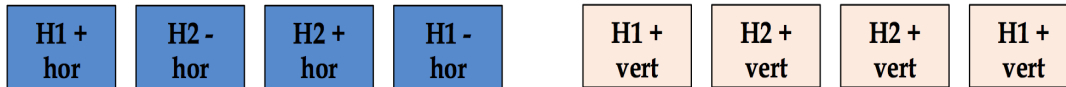
Figure 3.78: Rotator reconfiguration: The RHIC spin rotators (blue) consist of four helical magnets of different helicity with horizontal field at the magnet entrance. The sign demonstrates the magnet helicity: “+” is right-handed, “-” is left-handed (shown in the left side of the picture). The RHIC Siberian Snakes (pink) consist of four helical magnets of the same helicity with vertical field at the magnet entrance. Reconfiguration of a spin rotator into a snake can therefore be accomplished by a 90^\circ rotation of the helical magnets.
