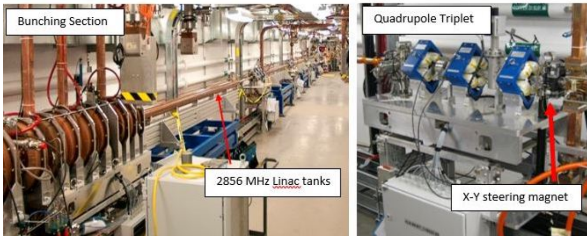
Figure 3.133: Continuous solenoidal field coils and quadrupoles from NSLS-II LINAC.
