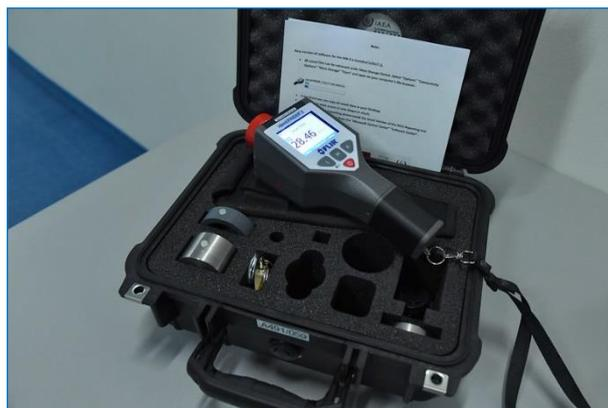
Figure 19: A radionuclide detector, the Hm5.
