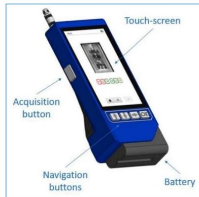
Figure 44: Prototype of a unified seal reader under MSSP Task EC E 2008 (Identification, Development, Testing and Vulnerability Assessment of Sealing Technologies for International SG).
