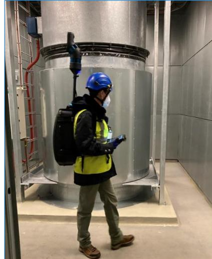
Figure 72: A Department staff member conducting 3D mapping of a facility using LiDAR sensors as part of a Design Information Verification (DIV) activity.
