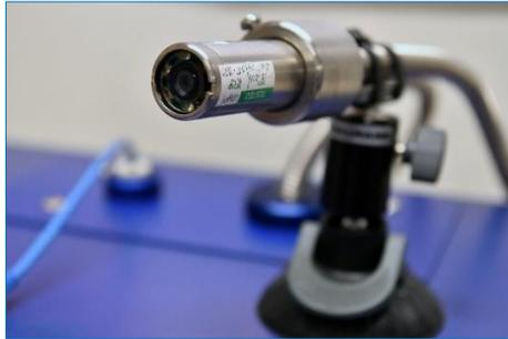
Figure 49: A radiation-hardened camera connected to NGSS DCM-A1 modules.
