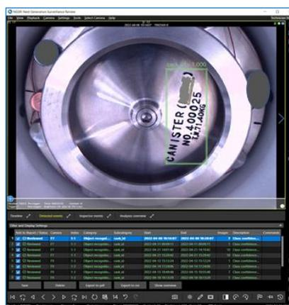
Figure 71: Test of integration of deep learning algorithms within NGSR to enhance surveillance review capability.
