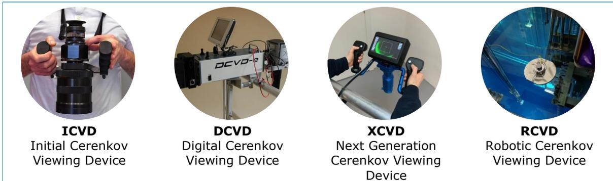
Figure 52: Evolving Safeguards Instrumentation: From ICVD to RCVD – Four Generations of Cerenkov Viewing Devices.
