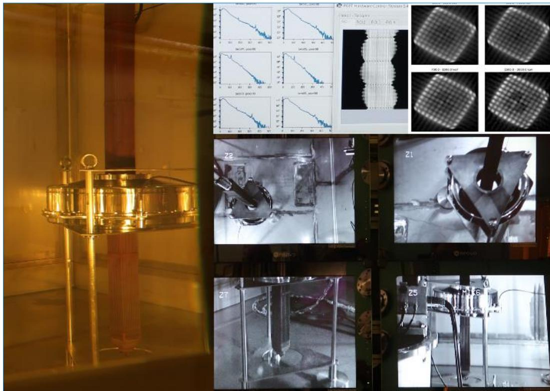
Figure 74: The Passive Gamma Emission Tomography (PGET) system's performance evaluation on the Boiling Water Reactor (BWR) spent fuel in a hot cell at Zwiilag (Switzerland).
