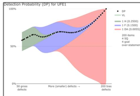
Figure 68: This is a detection probability graph produced by SAMPLAN, which shows the range of how much the detection probability would change with the addition or removal of one measurement -this shows the sensitivity of detection probability to small changes in the sample size.
