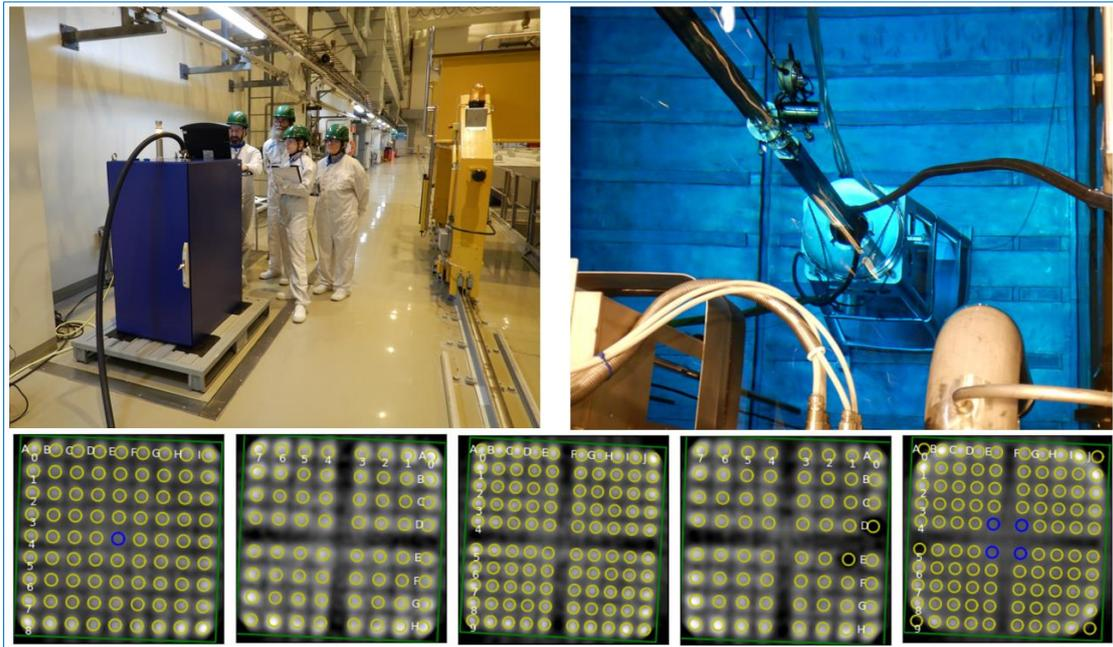
Figure 73: Testing of the Unattended Gamma Emission Tomography (UGET) at the interim Spent Fuel Storage at the Olkiluoto Nuclear Power Plant (Finland).
