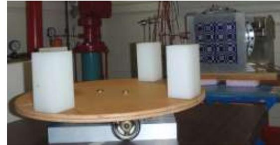
four Cf-252 sources embedded in polyethylene blocks
