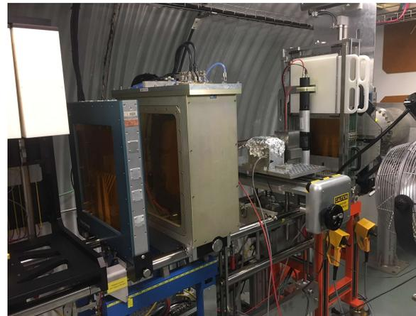
Left: Integrated 10-module CdZnTe calorimeter prototype
