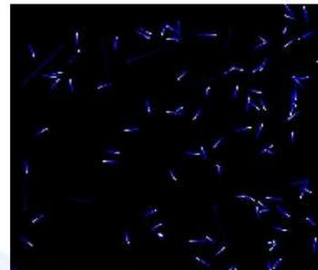
Color scaling reflects 6-bit digitization of amplitude of pad charge signal.
