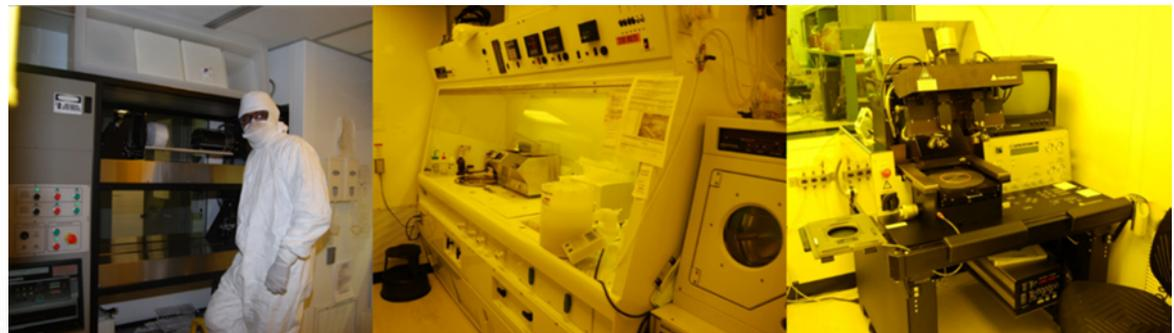
Pictures of the class-100 Clean room for the silicon processing.
