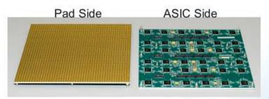
5mm × 5mm Pad size: 24cm × 24cm Pad board:  $48 \times 48 = 2304$ # pads: # layers: 11 Board thickness: 2.8 mm (0.011") ASIC 64 channels #ASICs 36 Brookhaven Science Associates
