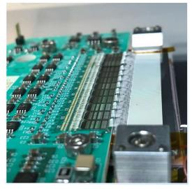
384-strip germanium detector wire-bonded to 12 MARS ASICs
