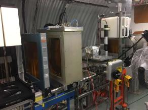
Left: Integrated 10-module CdZnTe calorimeter prototype Right: CdZnTe detectors in a radiation beam line at NSRL
