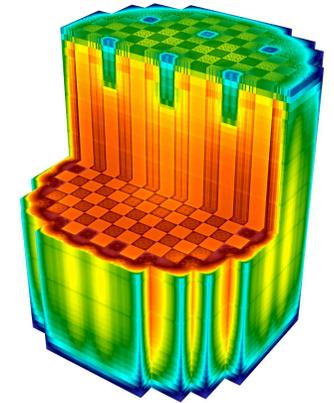
A visualization showing the distribution of the fission product Xenon-135, an important marker for predicting reactor behavior, in the WB2 reactor core during startup. VERA enables the detailed tracking of Xenon-135 with greater fidelity than any modern reactor simulation tool available today. From ORNL
