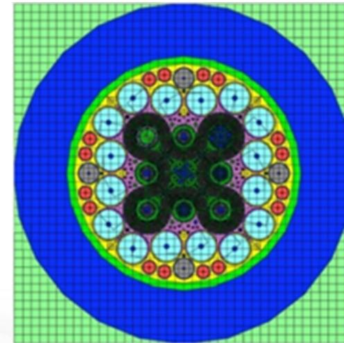
SCALE model of INL Advanced Test Reactor
