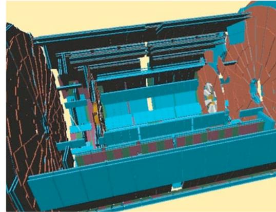
ATLAS detector muon system, simulated in GEANT4
