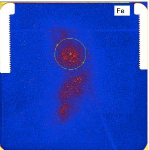
10x10 cm swipe sample Loaded with NIST # 2584, indoor dust sample with added U particles.
