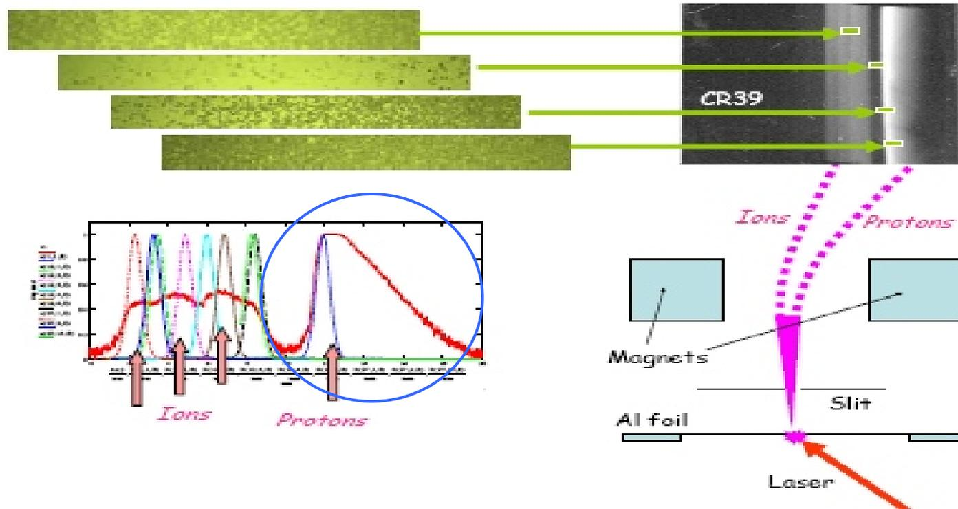
Proton and ion energies were diagnosed with a compact magnetic spectrometer followed by a CR39 plate. A density plot obtained with a scanner is overlaid with artificial peaks that illustrate the expected position and spread due to a finite spectrometer slit for the 1-MeV protons and any possible Al<sup>+n</sup> and C<sup>+n</sup> ions accelerated in the same field.
