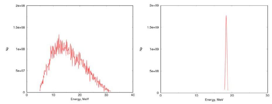
Fig. 8 Proton energy spectrum from a structured target. (a) Solid state laser with λ=1μm. (b) CO<sub>2</sub> laser with λ=10μm. The CO<sub>2</sub> laser produces a much narrower proton spectrum because of the narrower phase space fill.
