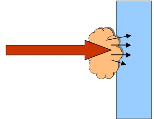
**Stage 2.** Relativistic electrons propagate through the target and form a dense cloud behind it
