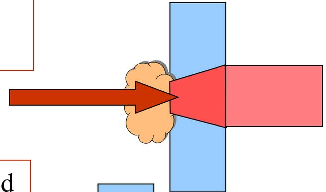
**Stage 3.** Electron cloud and the positively charged target create electric field ( $\sim 10$  GV/m), which ionizes atoms of the target back surface and pulls ions (protons) out, accelerating them
