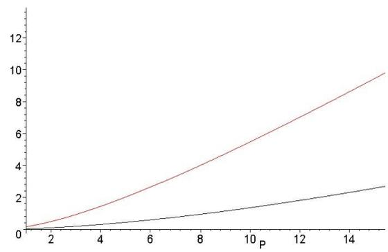
**Proton energy (MeV) vs laser power (TW). Red is for 10 μm, blue is for 1 μm**
