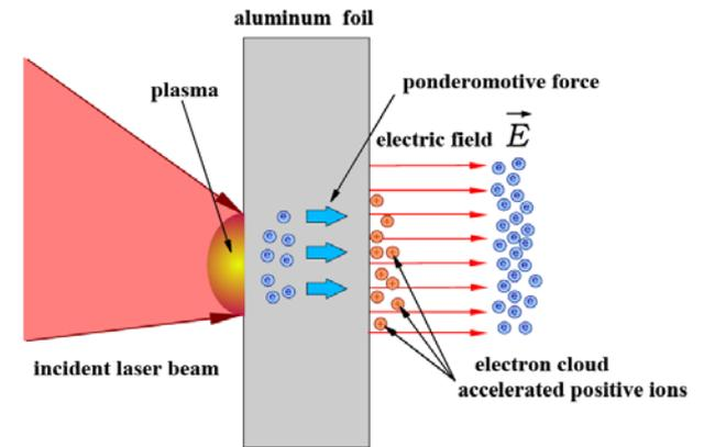
**TNSA the main mechanism until high intensity  $10^{23} \text{ W/cm}^2$**
