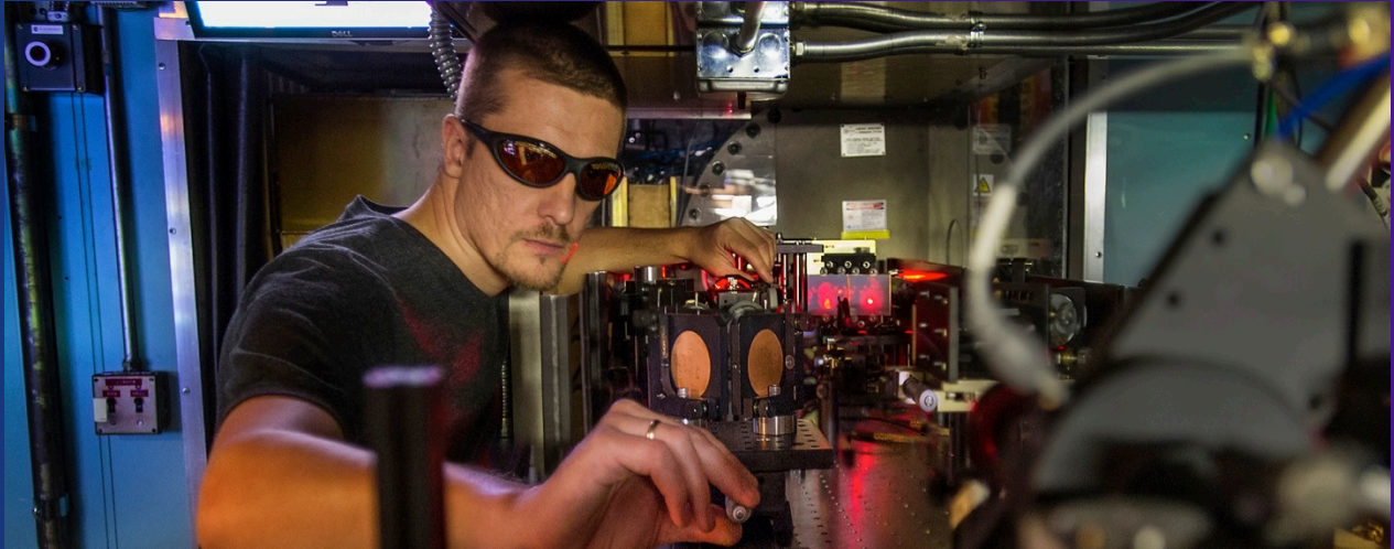
ATF laser physicists, Mikhail Polyanskiy, works on alignment of the first ever mid-IR CPA compressor.
