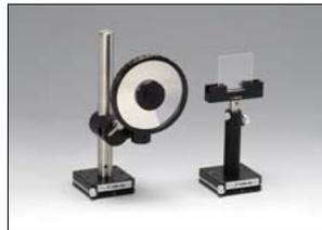
The adjustment tool of input light intensity for C1808-03. A variable ND filter and a laser beam splitter are included.
