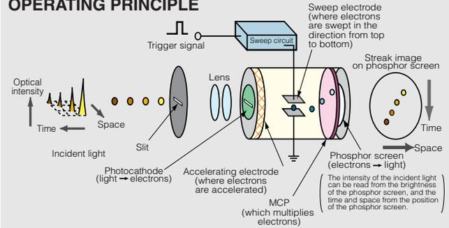
The light pulse to be measured is projected onto the slit and is focused by the lens into an optical image on the photocathode of the streak tube. Changing the temporal and spatial offset slightly each time, four light pulses, each with a different light intensity, are introduced through the slit and conducted to the photocathode.
