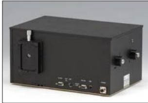
The combination with streak camera enables to measure wavelength, time and light intensity simultaneously.
