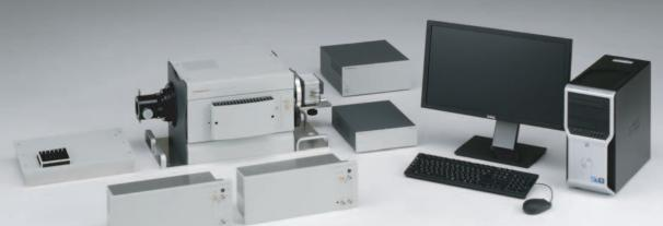
The C10910 streak camera includes a choice of streak tube detectors and a variety of plug-in options for optimum performance.
