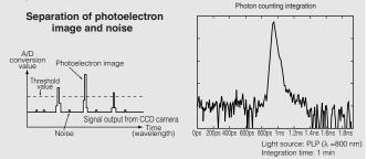
Positions in the photoelectron image which are above the threshold value are detected and are integrated in the memory, enabling noise to be eliminated completely. This makes it possible to achieve data measurements with a high dynamic range and high S/N
