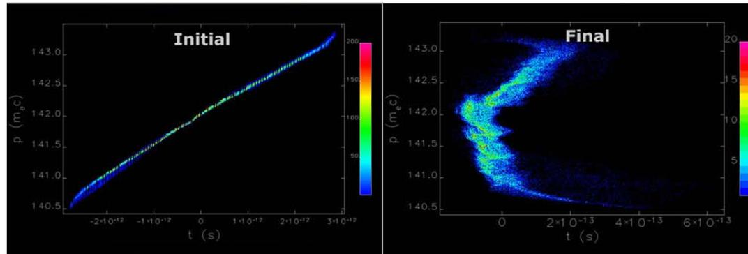
Parmela-Elegant simulation longitudinal phase space of beam, with compression from 50A to 1.5 kA.
