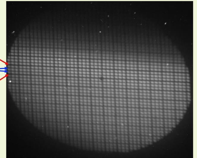
Shadow of the TEM grid (square thick/thin 30 $\mu\text{m}$  opening/16-10-10 $\mu\text{m}$  bars) obtained using an improved e-beam imaging system.
