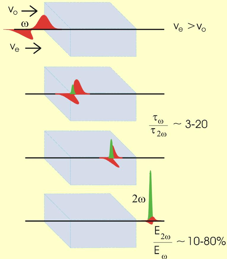
SNLO code simulations of 1064 to 532 nm conversion in 10 cm crystal with group velocity mismatch.
