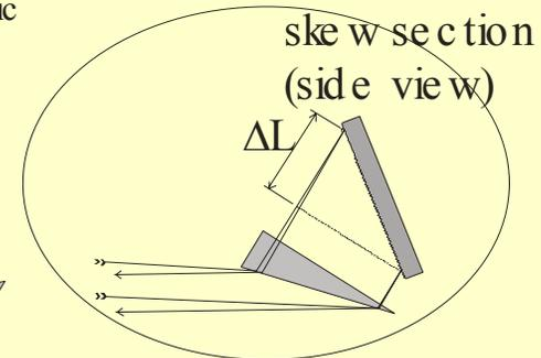
The transverse time delay is created by using a diffraction grating. The variation in path length across the beam produces a total range of  $2\Delta L/c$ .
