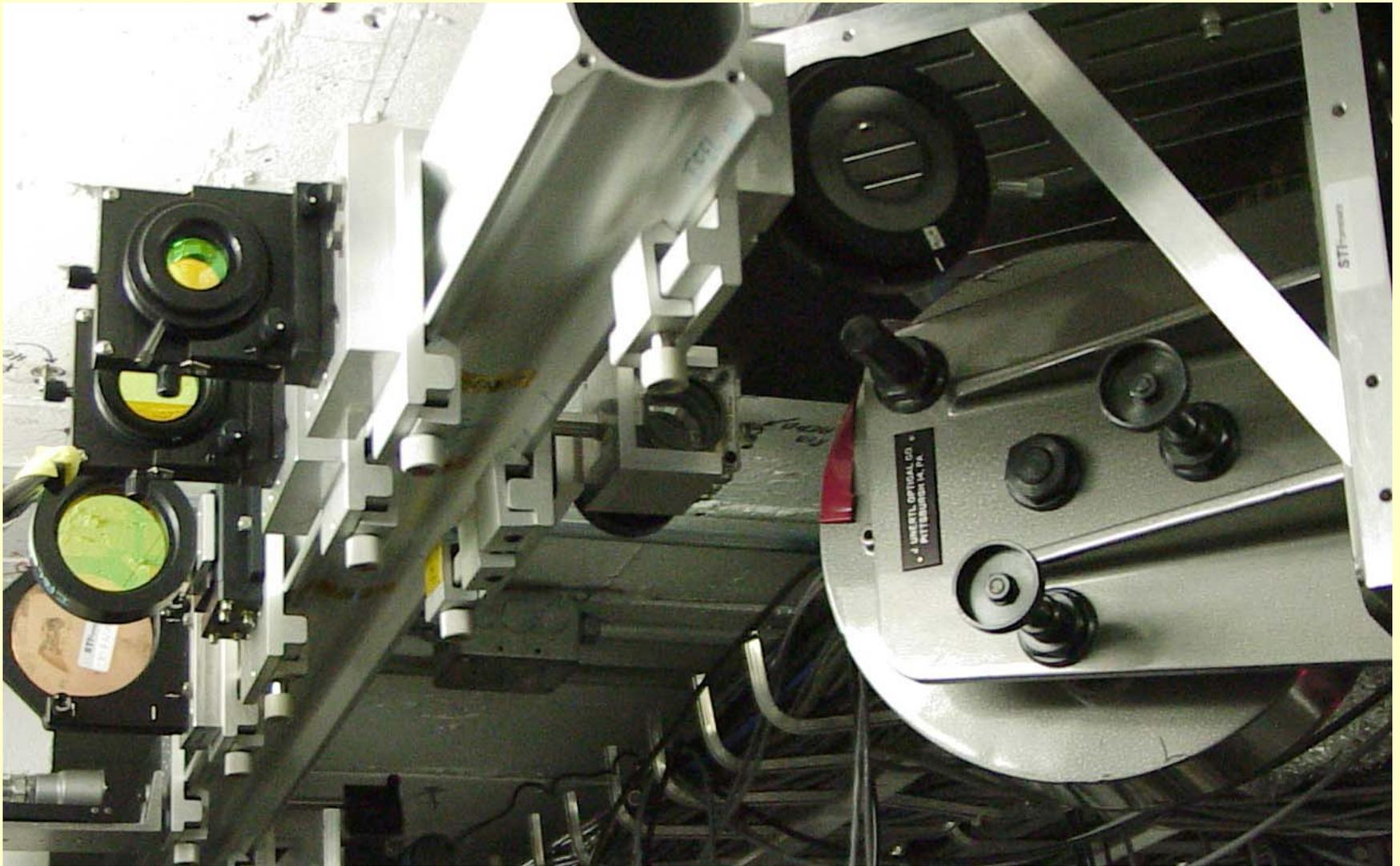
6-foot motorized optical delay stage
