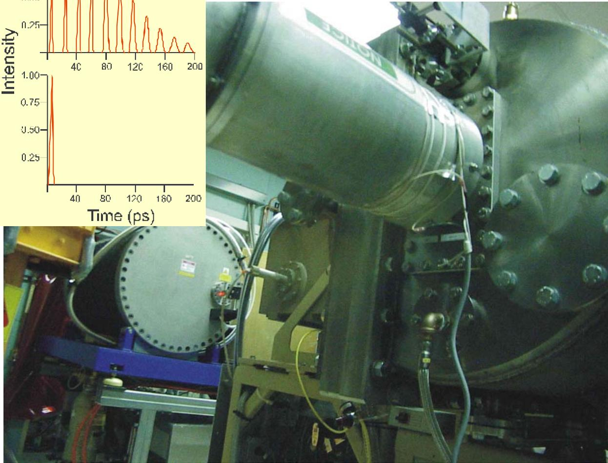
Final  $\text{CO}_2$  amplifier is upgraded with adding extra 2 passes (6 total) and external mirror adjustment
