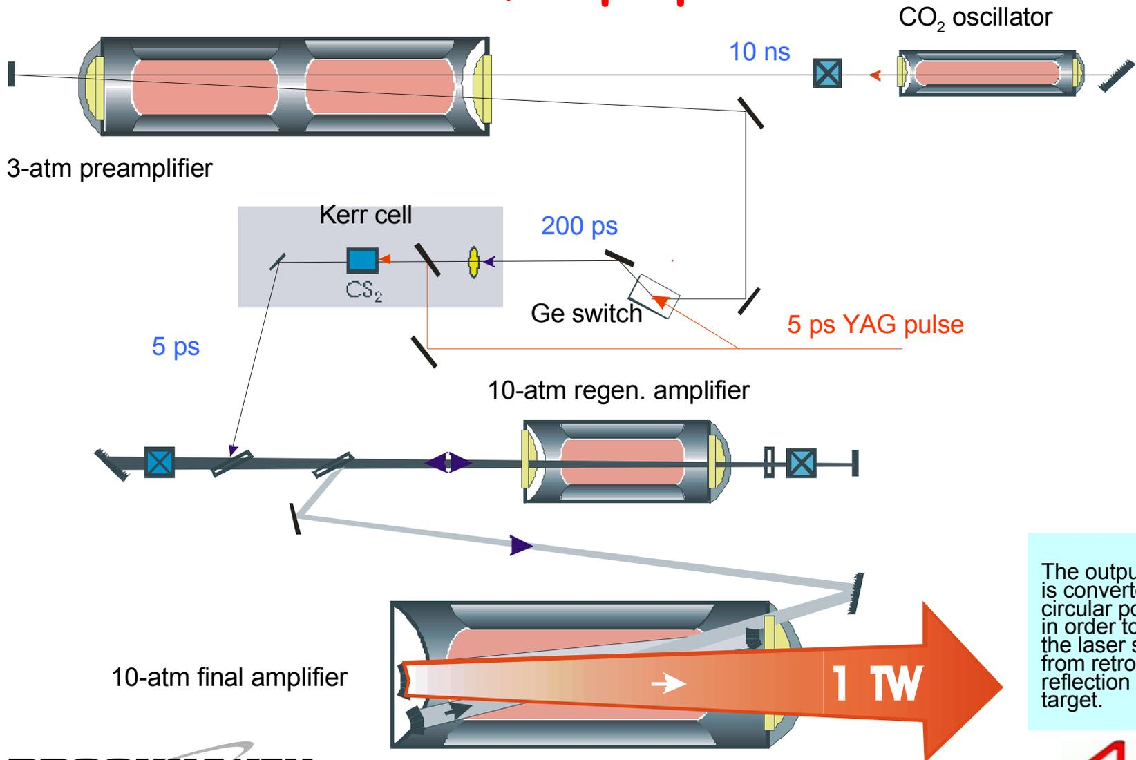
The output beam is converted to circular polarized in order to protect the laser system from retro-reflection from the target.
