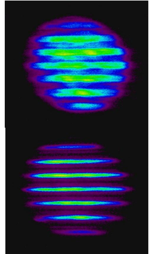
A micromirror array as used in commercial projectors is robust enough to serve as an active beam shaper for a laser beam.
