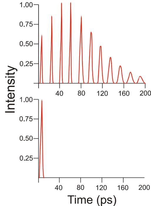
Strongly modulated rotational line structure of the  $\text{CO}_2$  gain spectrum modifies the frequency content of picosecond pulses, changing their temporal structure.
