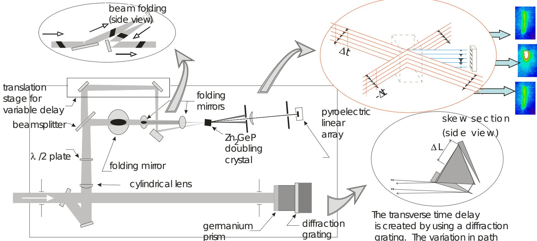
The transverse time delay is created by using a diffraction grating. The variation in path length across the beam produces a total range of  $2\Delta L/c$ .
